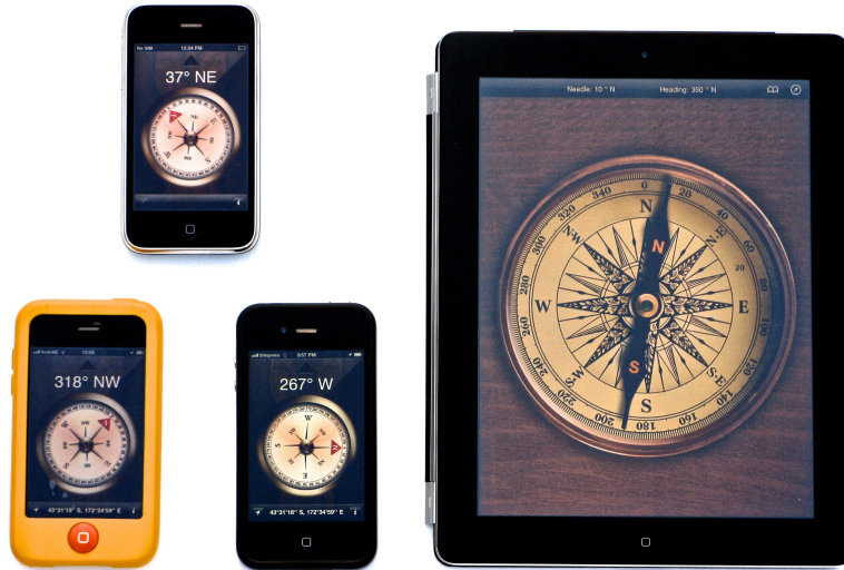
FIGURE 1.3: An example of sensor error in the magnetic compass: a variety of different devices are all measuring a different magnetic north. Ideally, they'd all be pointing in the same direction.
